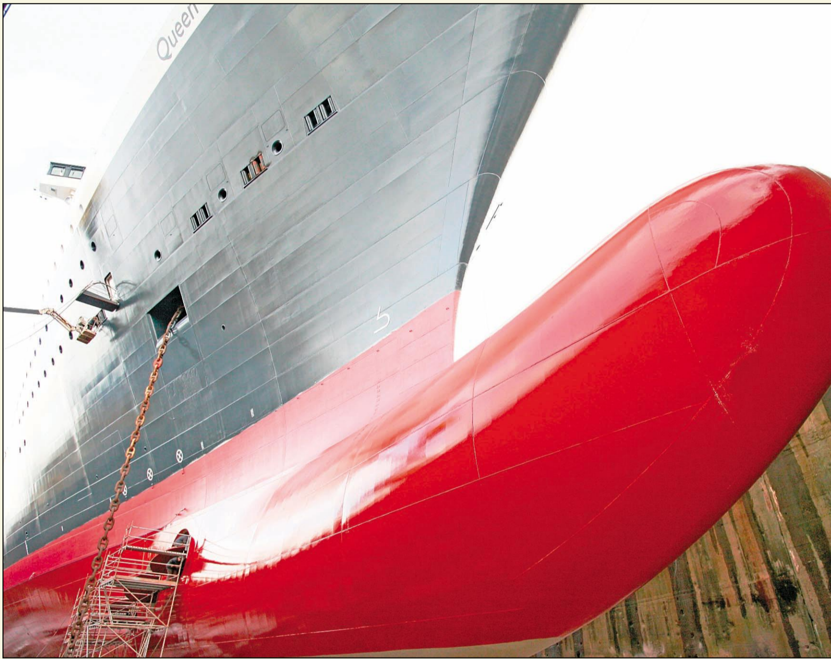
CUNARD Line's Queen Mary 2 had 6,000 sq m of hull blasted and recoated with a fluoropolymer foul-release coating from International Paint. The cruiseship recently completed a spruce-up at Blohm+Voss in Hamburg, ahead of the coming cruise season.
