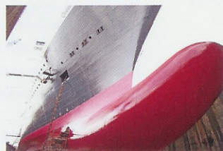
QM2 in drydock during application of Intersleek 900
