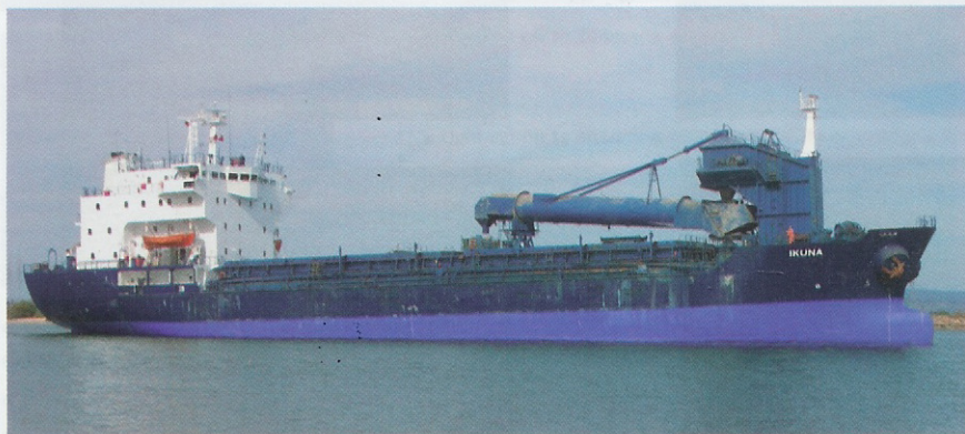
'Ikuna' has also benefited from Intersleek 900 foul release coating
