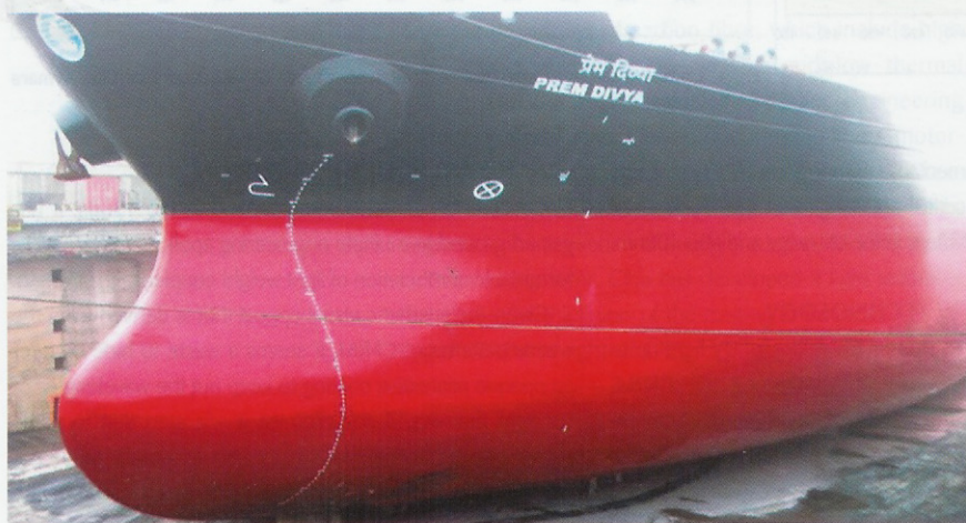
'Prem Divya' coated with International Paint's Intersleek 900
