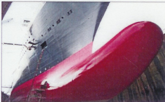
Conard Line chose International Paint's fluoropolymer foul release coating Intersteek 900 for the underwater hull of its transatlantic ocean liner Queen Mary 2.
