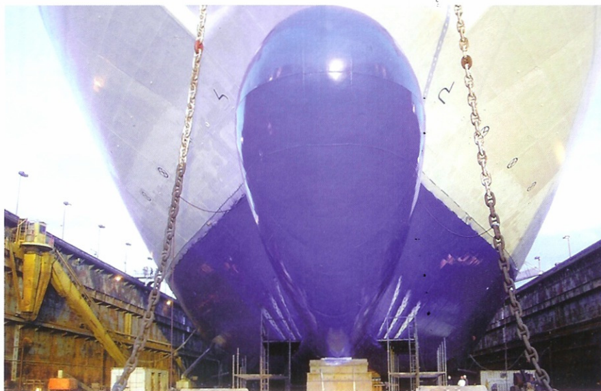
In late 2007, International Paint completed a hull coating project on Carnival Victory . The cruise vessel was coated with Intersleek 900 during drydocking in the Grand Bahamas Shipyard. A sister ship, Carnival Valor , was coated with the same product earlier this year.
