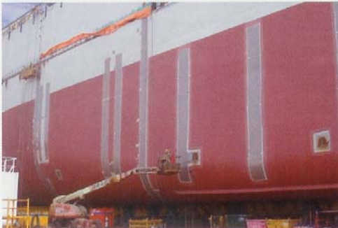
Intergard 787 primer, designed to limit VOC emissions, is applied to the exterior shell of a newbuilding
