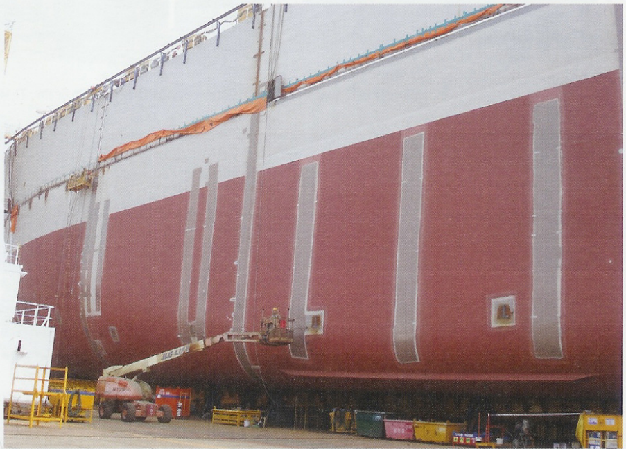
Intergard 787, outside shell at newbuilding (Credit: International Paint Ltd).
