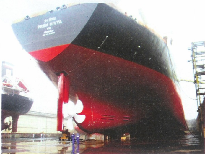
The tanker Prem Divya which has been coated with Intersleek 900
