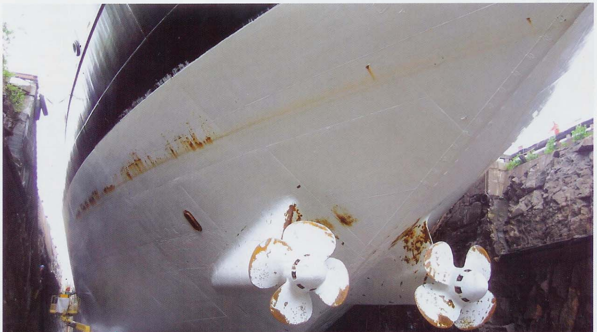
Intershield® 163 Inerta 160 after 60 months in service.
