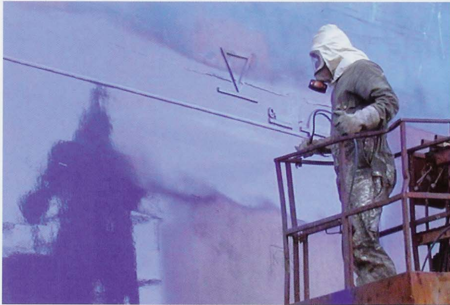
The first Classification Society recognised abrasion resistant ice coating was Intershield® 163 Inerta 160, from International Paint.
