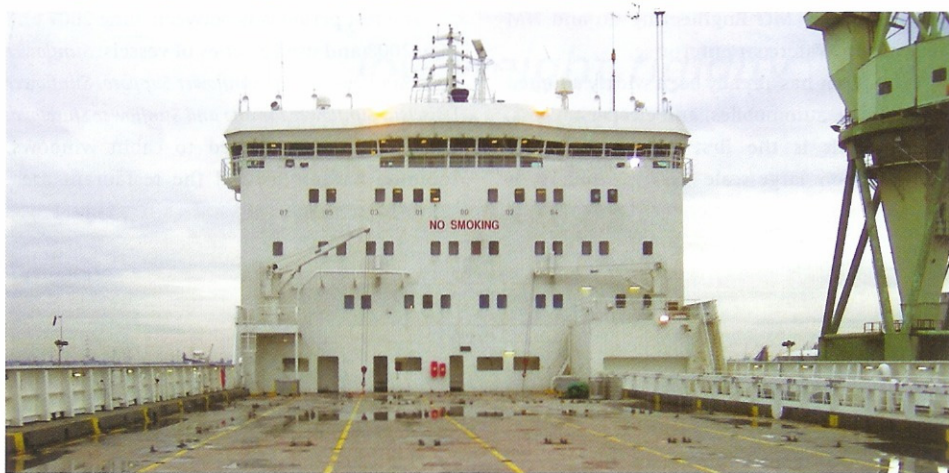
MC Technology's moisture cure urea coating is used for areas such as ro-ro decks
