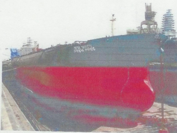
Aframax Tanker 'Prem Pride'. At corresponding engine speeds, the vessel was consuming up to 6% less fuel after the application of Intersleek 900
