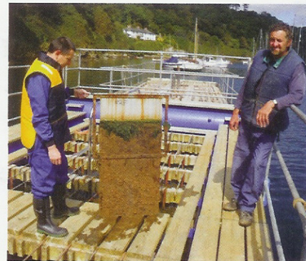
A fouling reference board being inspected
